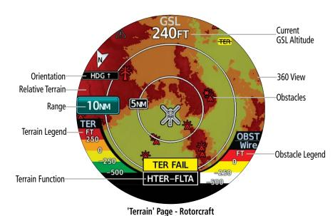
When Terrain-FLTA or TAWS-B data is available, potential impact areas will be indicated. If an obstacle and the projected flight path of the aircraft intersect, the display automatically adjusts the range setting to emphasize the display of the potential impact area.
