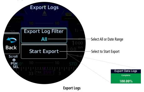
All flight data logged on a specific date is stored in a file named in a format which includes the date, time, and nearest airport identifier.
