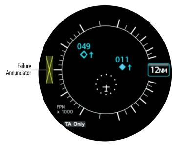
**Vertical Speed Failure Annunciations**
