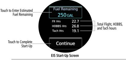
**NOTE:** The EIS Start-up Screen will not be displayed if the GI 275's system believes the aircraft is airbone and/or during the previous power cycle, the system was shut down in an airborne logic state.
