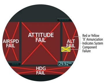
**Example of Failure Annunciations**
